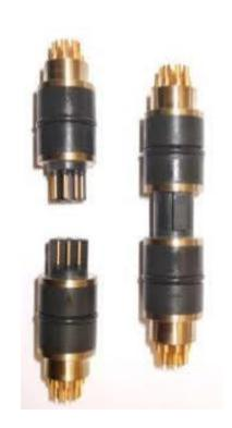
LK16664 4 Pin / 6 Socket LK16665 6 Pin / 4 Socket Medium Pressure/Medium Temperature Connectors Rated to 170°C, 10,000psi
